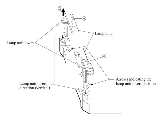
Figure 5.6 Lamp unit replacement
